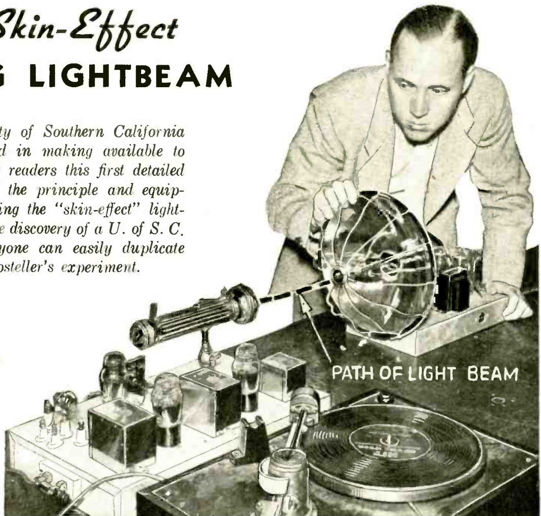
Gerald Mosteller, University of Southern California graduate, is shown with a portion of his apparatus for sending sound over a lightbeam, using an ordinary 5-cent flashlight bulb and simplified radio parts. His discovery formed the thesis for his Master's degree at the University.
